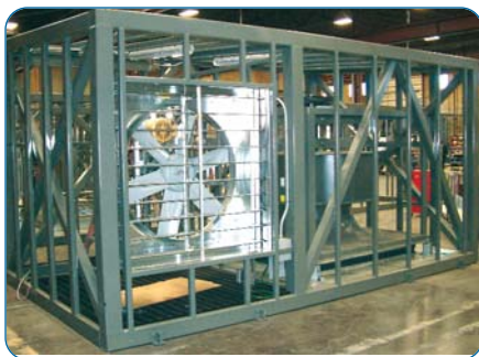
Top fan section with prop exhaust fan and vertical plenum supply fan. Fans, drives, power wiring and controls were all factory-installed, minimizing required site work.
