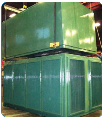
Two air handlers, each delivering 62,000 cfm, were designed to be stacked as four sections, simplifying transportation and site erection.
